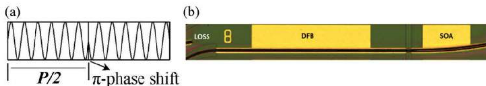
Fig. 1. (a) An sampled Bragg grating with two phase-shifted sections (2PS-SBG), P is the sampling period, (b) the micrograph of the fabricated device.
