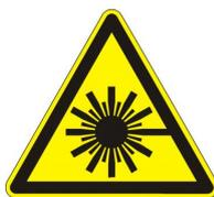
*For the area signs the specifications are quite simple - 50% of the area should be yellow and the width of the black border is 0.06 x the length of the side. A more detailed specification is given for the symbol used in labels, see spec on in BS EN 60825-1*
