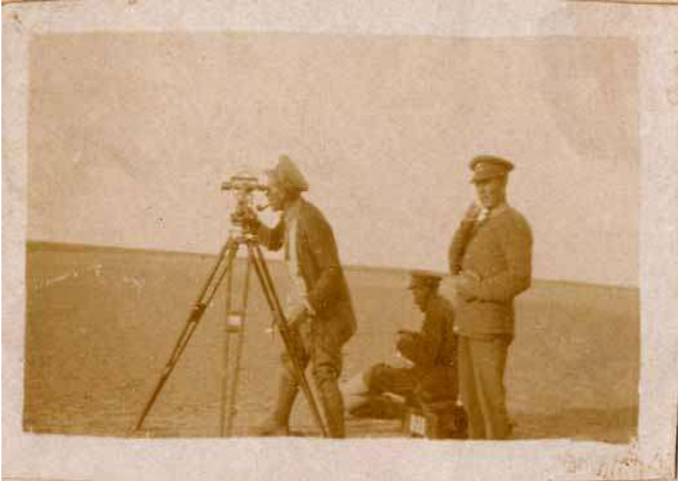
Using a theodolite in the Desert (Photograph loaned by Claud H. Williams's family.)
