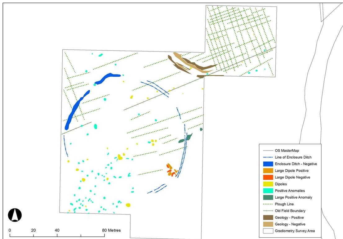
*Fig 5: Interpretive plot of the gradiometry results, showing the outline of the causewayed enclosure, and a series of dipole readings near the southern entrance gap (Poller 2013)*
