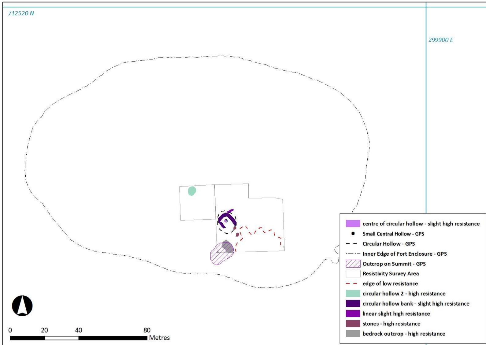
Figure 6: Interpretation of resistivity data and features on summit measured by GPS
