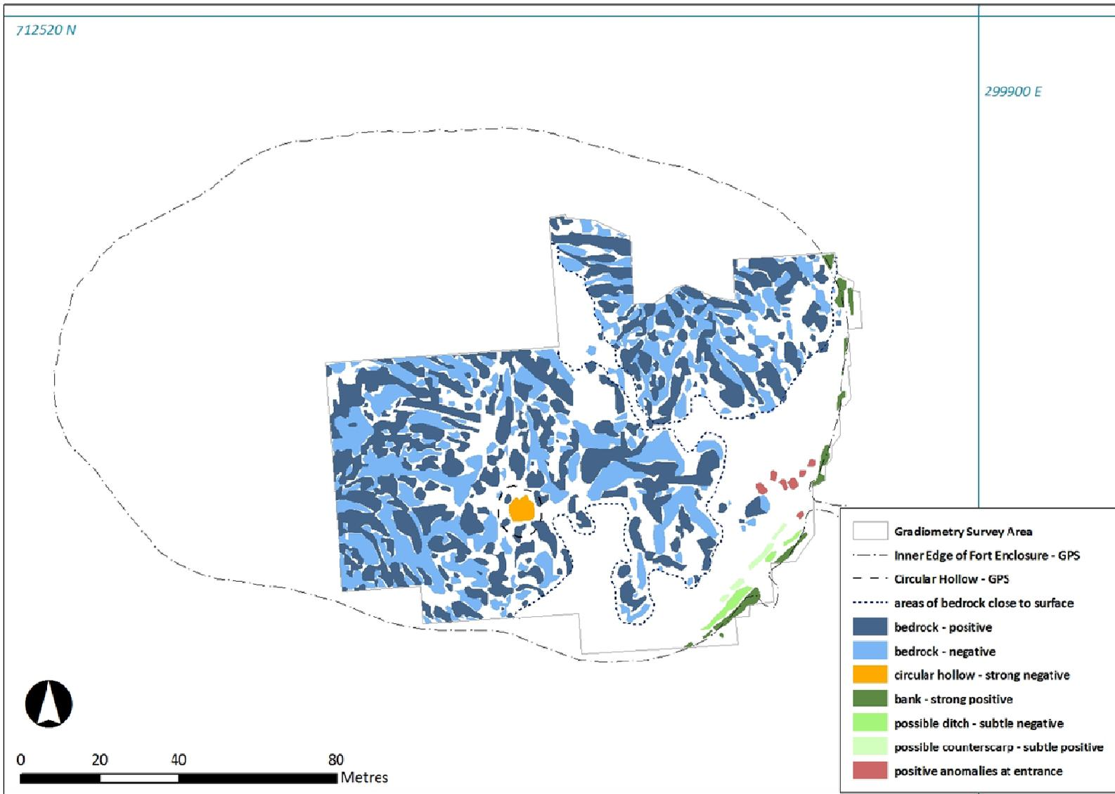
Figure 4: Interpretation of processed gradiometry data and location of hollow on summit mapped by GPS
