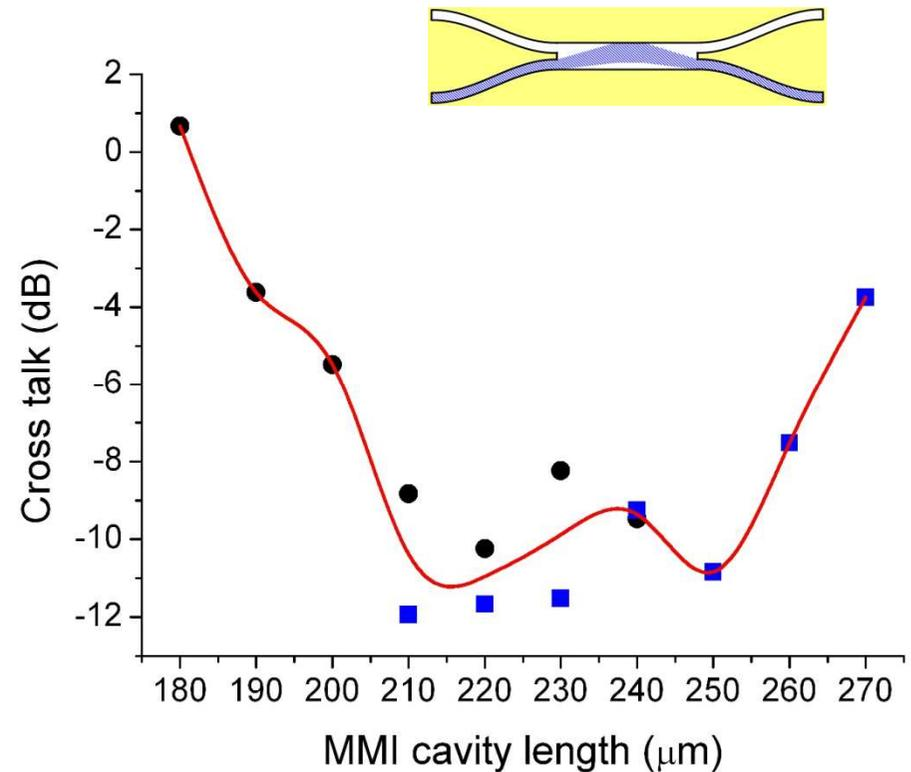
**Optimum coupler length  $\sim 220 \mu\text{m}$**
