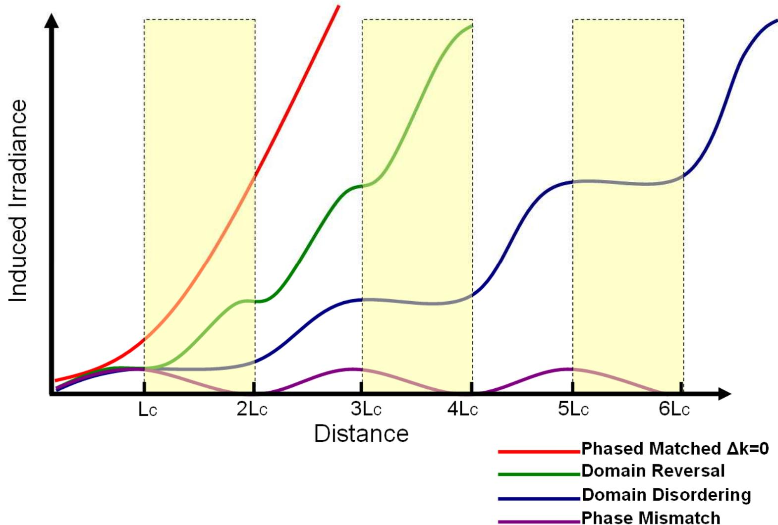
**The generated wave must remain in phase with the nonlinear polarisation source to build up to a substantive level**
