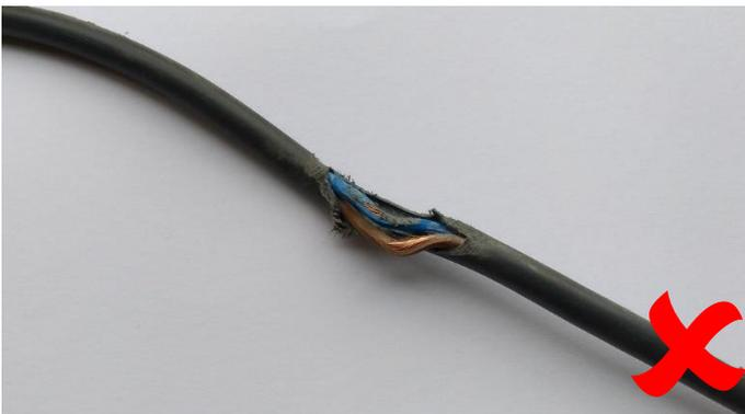
Flexes should be visually inspected and checked physically by running a hand along the length. If there are any breaks in the insulation the appliance should not be used.
