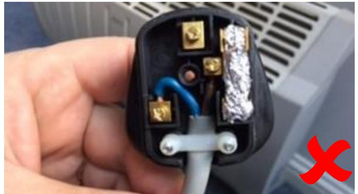
Plug fuses should be tightly fitted, correctly rated and should not be tampered with (e.g. by wrapping them in foil). Improvised fuses should never be used.
