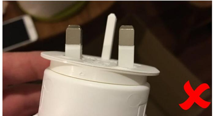
If any of the plug pins are bent, deformed, corroded or missing the appliance could pose a fire risk and should be removed from use.
