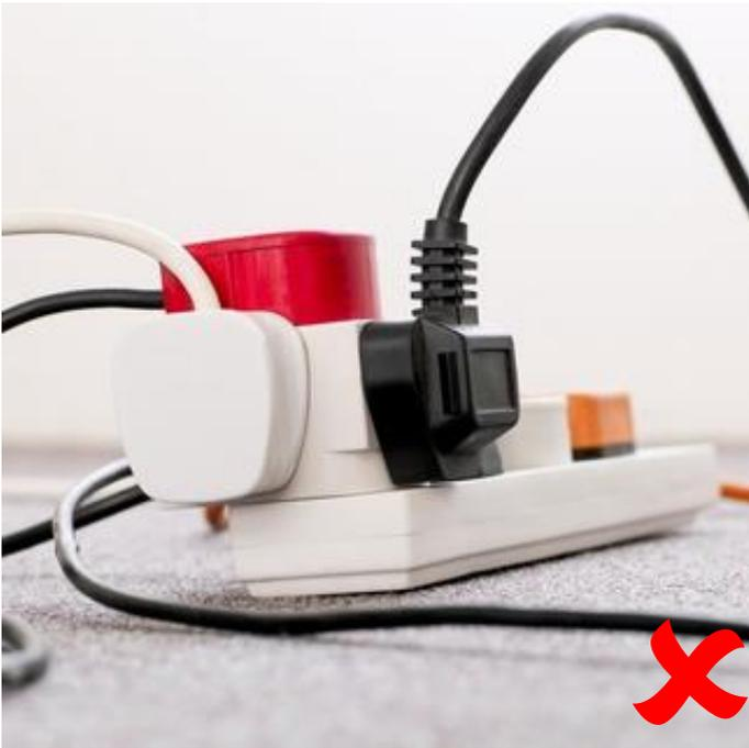
Avoid overloading extensions particularly if you are using appliances that require a lot of power such as heaters, remember most extensions are only rated to 13A. Overloading sockets can lead to an increased risk of electrical faults and fire. Remember that extensions should be subject to the same visual inspection as any other appliance.
