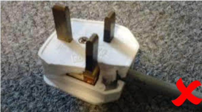
The casing of the plug should be in good condition with no cracks, chips or missing pieces. They should not be held together with tape.
