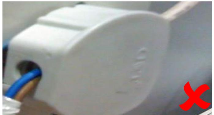
The outer insulation of the plug flex should be held by the cable grip. It should not be possible to see the insulation of the live, neutral or earth wires.
