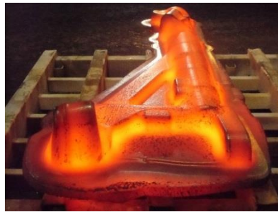
Forged CRES main fitting after closed die operation. (Courtesy of Aubert & Duval)
