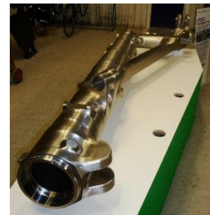
Fully machined CRES main fitting presented at TRL5. (Courtesy of Airbus)
