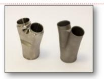
Additive layermanufactured pipe fittings 50% lighter
