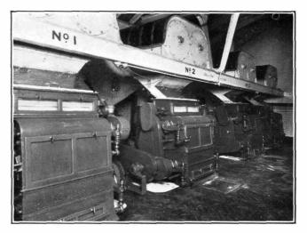
THE MILLS USED FOR GRINDING THE MALT
