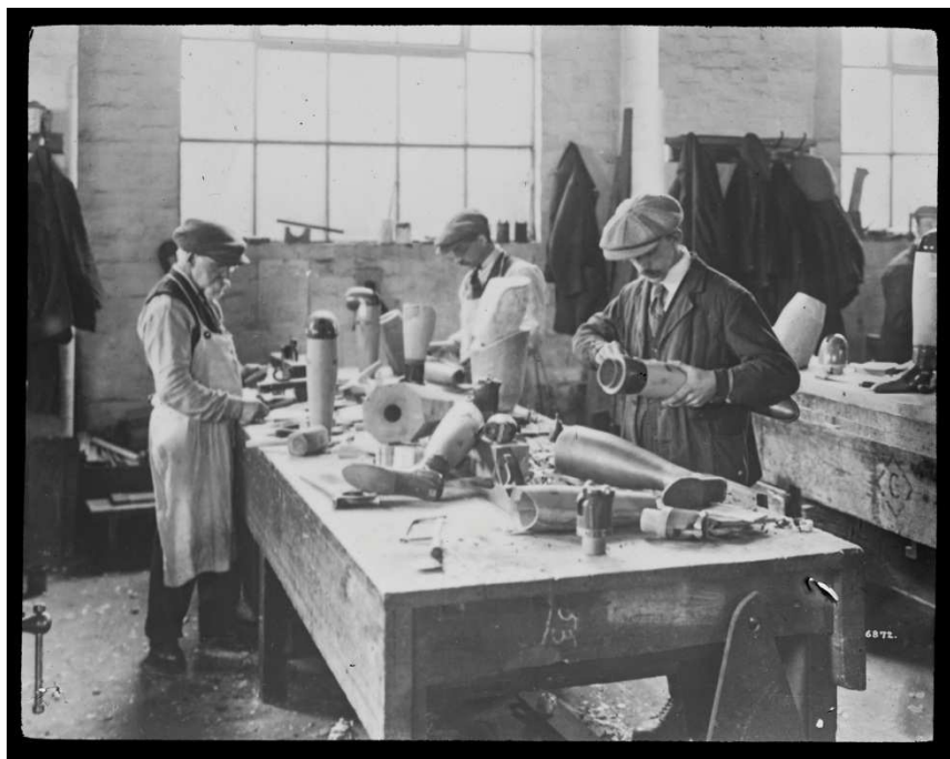
Figure 8 The manufacture of prosthetic limbs from the collection of Sir William Macewen held by the University Archives
