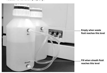
Fig. 12. Waste and sheath fluid bottle connections.
