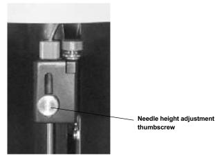
Fig. 16. Sample needle assembly.
