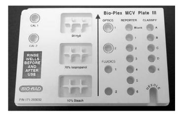
Fig. 8. Maintenance, calibration, and validation (MCV) plate III.
