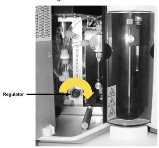
Fig. 20. Regulator screw adjustment.
