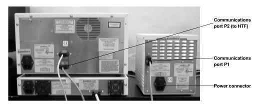
Fig. 7. HTF – rear panel view with connection to Bio-Plex 200 System.
