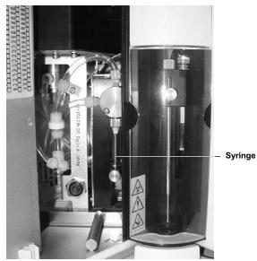
Fig. 3A. Sheath filter internal fluidics features.
