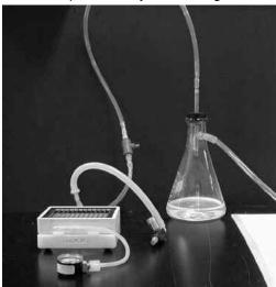
Fig. 21. Vacuum manifold and vacuum source setup.
