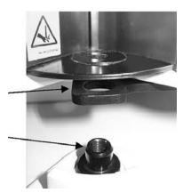
Fig. 10. Reader aligned on top of microplate platform.
