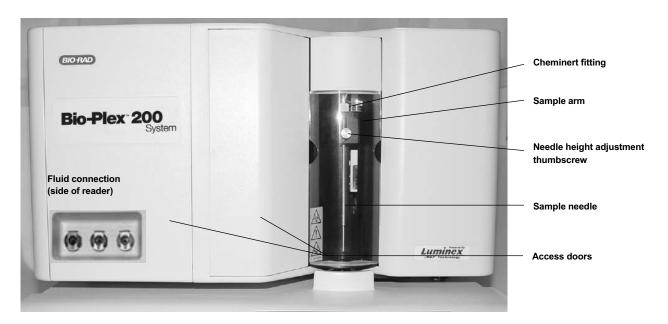
Fig. 1. Array reader – front and side panel features.
