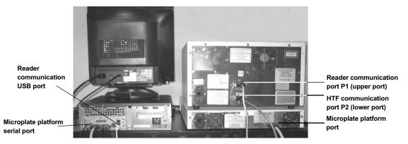
Fig. 11. Completed connections of computer and monitor to the Bio-Plex suspension array system.
