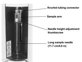
Fig. 14. Sample needle assembly.
