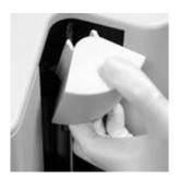
Fig. 13. Removing the light housing.
