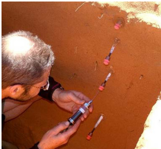
Gas sampling from a Kalahari 'soil' profile
