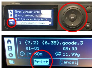
B – Use the down arrow button on the interface to move to the folder menu. Use the arrow buttons to find your file, and then press the “OK” button to select the file, and then to select “Print”.
