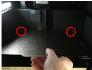
A – Ensure the magnetic build plate is keyed onto the platen and lying flat. Check that the build plate is clear of debris. If not, remove the plate and scrape debris away with the plastic scrapers provided. When done, carefully guide the build plate back on to the platen.
