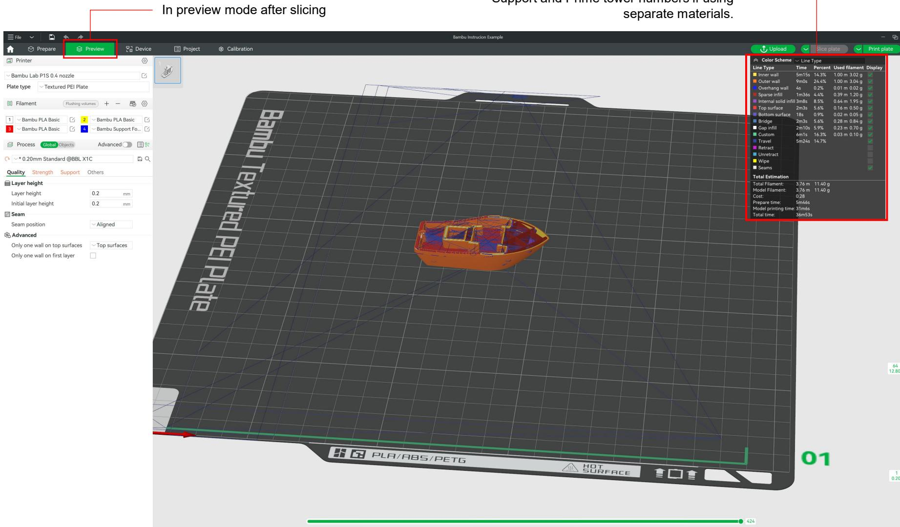
When selecting “Line Type” from the Colour Scheme drop-down, it is possible to see the time and material usage for different print operations of the build. It is important to pay attention to Support and Prime tower numbers if using separate materials.
