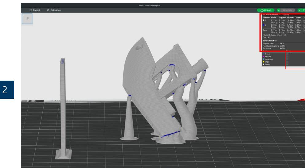
Note: Two filaments being used, and time estimation and material used. More changes = more time & material waste
