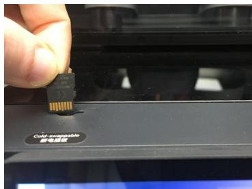
**A – The printer's MicroSD cards are cold swappable, meaning either the machine must be switched off OR the card safely ejected when it is removed, to avoid file corruption.** The switch to turn the printer off is on the back of the machine, right side when facing. Press the buttons on the LCD screen as shown in picture 2 to eject the card safely (do not click format card).
