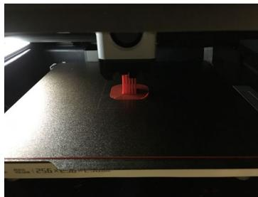
C – Wait at the machine until the start up procedure has completed and the **first layer of material has successfully printed**. This will take a few minutes. **Caution: the bed and nozzles heat up and become hot to touch during printing. Do not place your hands inside the printer once printing has commenced, as the printer head is in motion.** Options to pause/abort the print must be used if problems are noticed or wanting to interact with a model mid-print.
