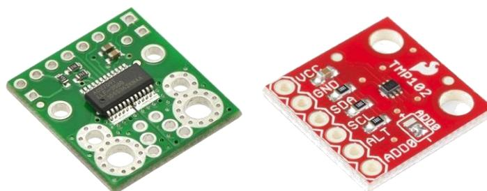
Fig. 8. Sensors for a) current ACS709  $\pm 75A$  [8] and temperature TMP102 [9]
