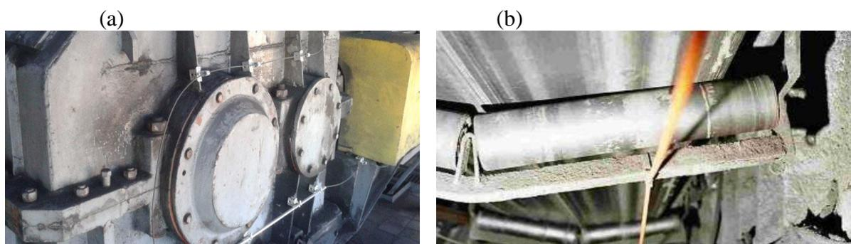
Fig. 1. Fibre optic temperature measurement (a) at the gearbox bearing and (b) along the conveyor [6]
