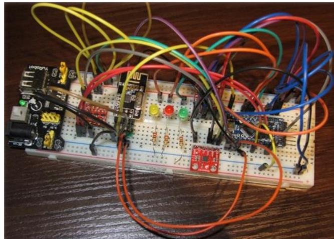
Fig. 10. Prototype of the measurement node responsible for the measurement of accelerations
