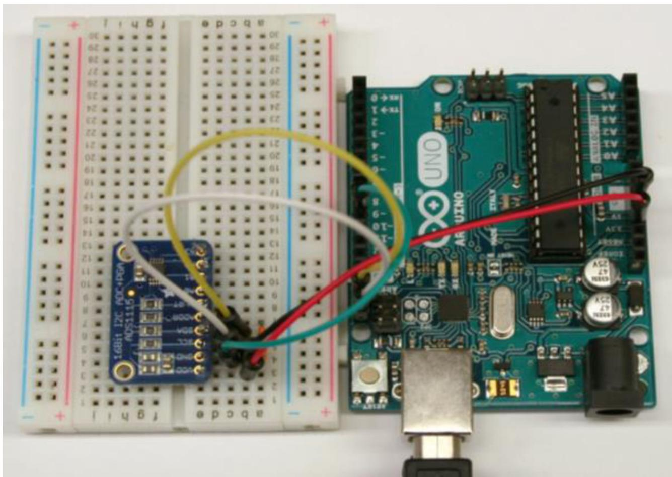
**Figure 1.** Photograph of the Arduino Uno, ADS1115 Analog-to-Digital Converter placed onto a circuit breadboard, and the wiring connections needed for the data acquisition device.
