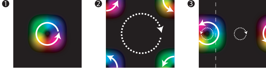
Fig. 5. Schematic of the transverse momentum density in different unit cells of the array shown in Fig. 2. Solid arrows indicate the momentum density in the beam. Comparison of cells ‘1’ and ‘2’ shows that in different unit cells the bulk of the momentum density can be at different radii from the cell’s centre (as the OAM in each unit cell is intrinsic and therefore independent of the axis position, we might as well calculate it with respect to a symmetric choice of axis position, namely the centre of the unit cell), leading to a larger OAM density according to Eq. (2), and that the circulation of the momentum density with respect to the axis (dotted arrow in ‘2’) can even be reversed, resulting in OAM of the opposite sign. The respective OAM per photon in unit cells ‘1’ and ‘2’ is 0.96\hbar and -2.93\hbar . In cell ‘3’ the OAM in each of the two parts of the cell (separated by the dotted white line) is intrinsic and equal and opposite that in the other part (the circulation of the momentum density in opposite directions is again indicated by dotted arrows), so the OAM in the whole cell is 0.
