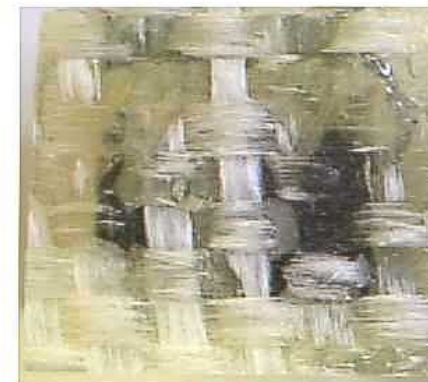
Interlaminar failure (polyester)
