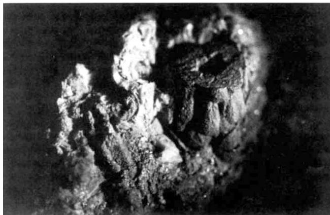
Fig. 1 Example of a 360-Myr old hydrothermal chimney from the Silvermines Zn+Pb+Ba deposit (8 mm chimney diameter).
