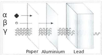
Illustration of the relative abilities of three different types of ionizing radiation to penetrate solid matter. Typical alpha particles ( $\alpha$ ) are stopped by a sheet of paper, while beta particles ( $\beta$ ) are stopped by an aluminum plate. Gamma radiation ( $\gamma$ ) is damped when it penetrates lead. Note caveats in the text about this simplified diagram.
