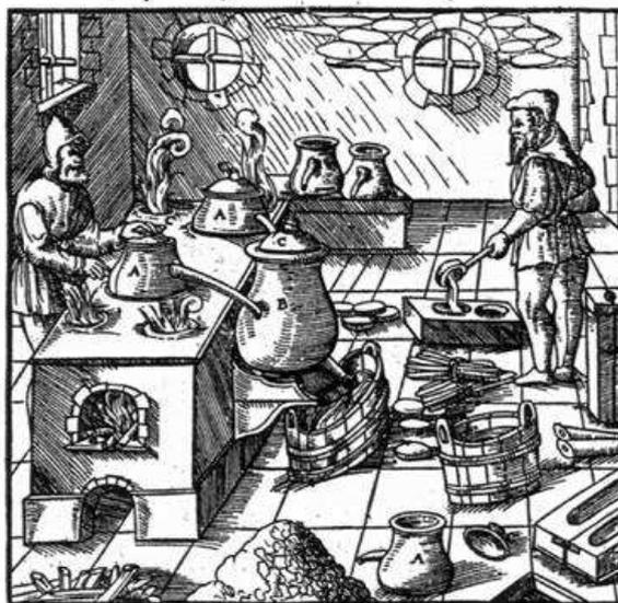
FIG. 24. Sulphur refining (Agricola, 1556).
