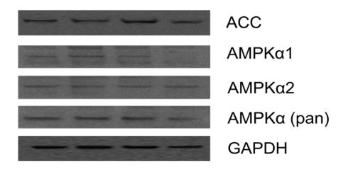
**Appendix D** - Western blot of control (AMPK<sup>+/+</sup>) mouse aorta and PVAT -/+ treatment with AICAR. Phospho-specific secondary antibodies detected by means of chemiluminesence.
