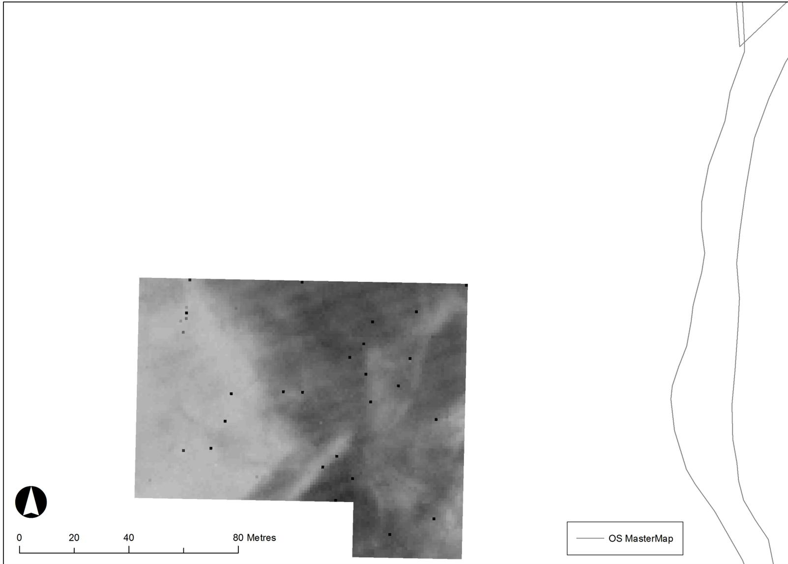
*Figure 6: Raw resistivity data*
