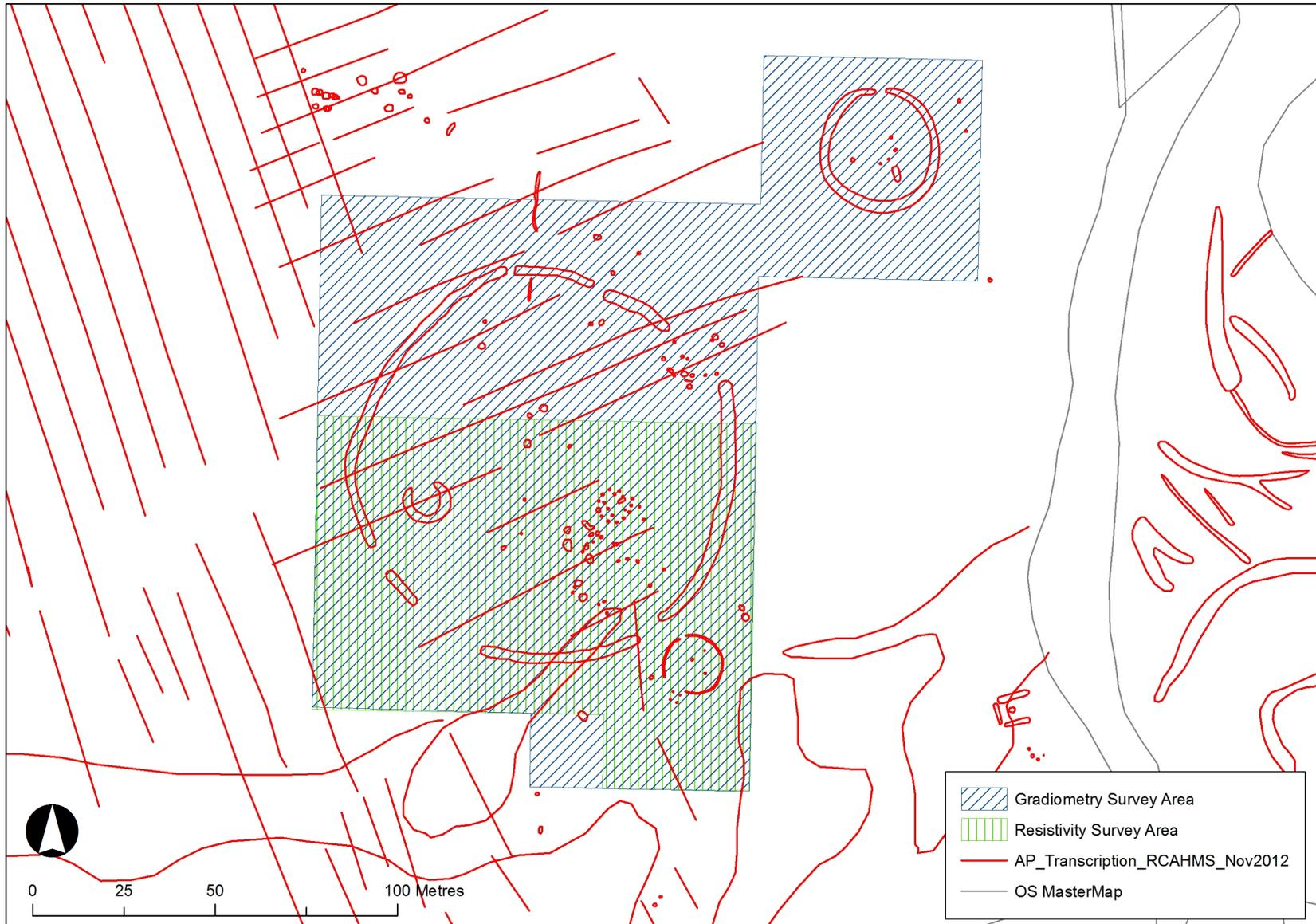
Figure 2: Location of the geophysical survey areas overlain on Ordnance Survey mapping data
