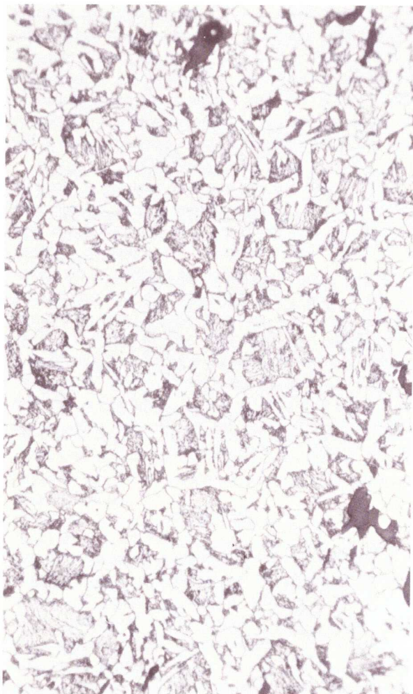
Fig. 49. Sword Inv. Nr. 833. Ferrite grains of widmanstätten structure with pearlite. Scale 400:1
