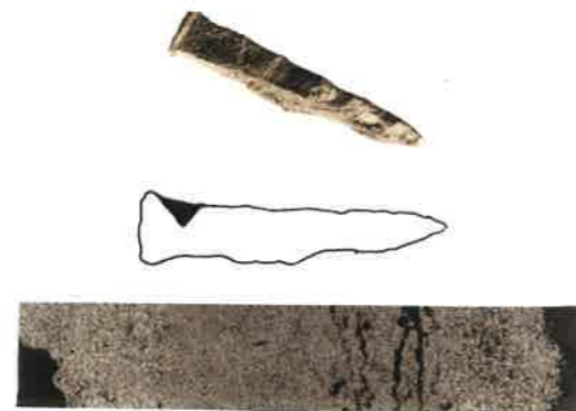
FIGURE 4. LB30 A1980.575 FERRITE WITH SPHEROIDISED PEARLITE. THE OBJECT HAS BEEN WELL AND EVENLY CARBURISED THROUGHOUT.
