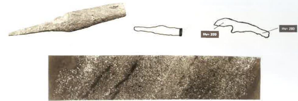
FIGURE 6. LB23 A1980.576, AWL OR CHISEL MARTENSITE UNIFORMLY DISTRIBUTED THROUGHOUT. FROM LEFT TO RIGHT: TOP: OBJECT; PLACE OF SECTION REMOVED; MICRO-HARDNESS MEASUREMENTS AT TWO DIFFERENT SPOTS ON THE SECTION; BELOW IMAGE OF SECTION (MARTENSITE).
