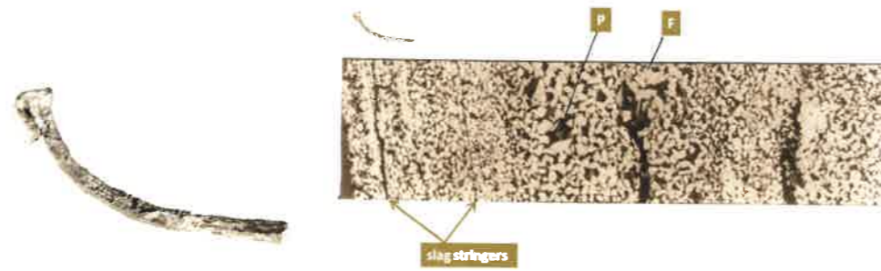
FIGURE 1. LB17 A1980. 621. P=PEARLITE; F=FERRITE; SLAG INCLUSIONS ELONGATED ALONG THE LINE OF WORKING. HARDNESS VALUES FOR THE TWO AREAS AND AT THE PEARLITE PHASE ARE: SMALL GRAINS HV=234, LARGE GRAINS HV=243.
