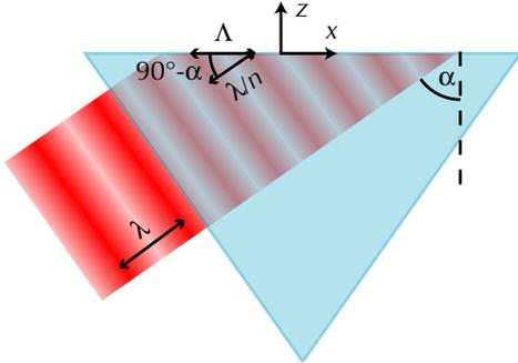
Fig. 1. (Color online) Geometry of the creation of evanescent waves by total internal reflection of a prism surface. A plane wave of vacuum wavelength  $\lambda$  is incident on a prism surface with angle of incidence  $\alpha$ . The transverse wavelength along the prism surface,  $\Lambda$ , is given by the equation  $\Lambda \sin(\alpha) = \lambda/n$ .
